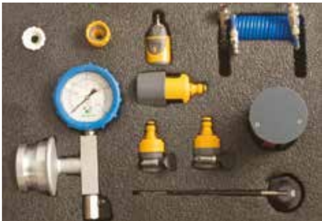
Flow and pressure test kit To take flows and pressures from taps and standpipe outlets
