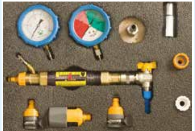
Levels of service flow and pressure To take flows and pressures from meter chambers and consumers outlets.
