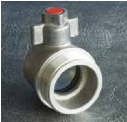
2 1/2" female instantaneous light alloy coupling x 3" BSP male thread.
