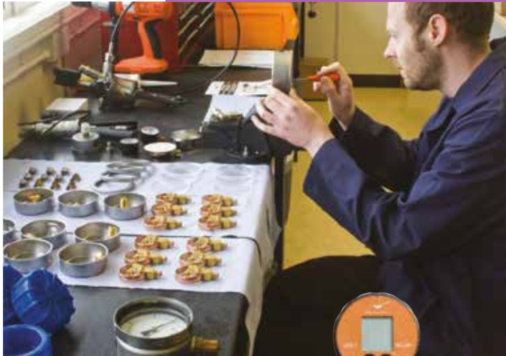
Digital Test gauges for accurate calibration comparison of Pressure and Vacuum instruments.
